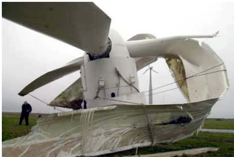
Figure 18. Structural collapse of a wind turbine in a 2002 storm. Source: Der Spiegel, DPA.
