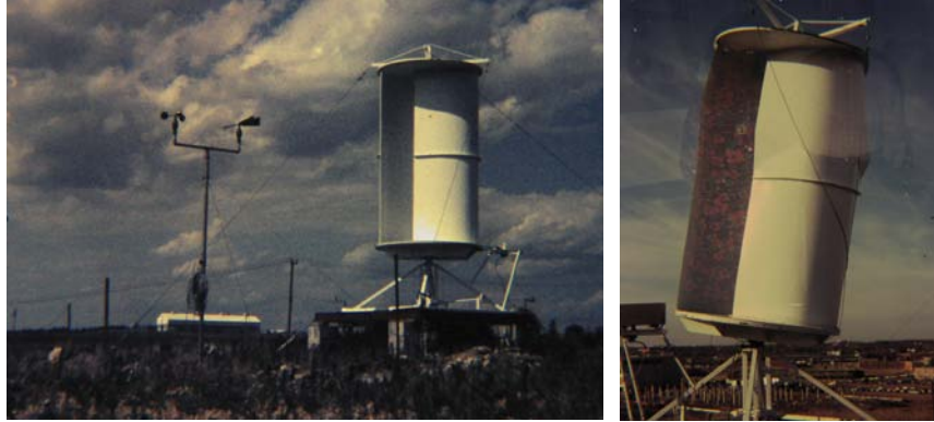
Figure 4. High winds damage effect on an experimental Savonius design wind turbine at Kansas State University, KSU.
