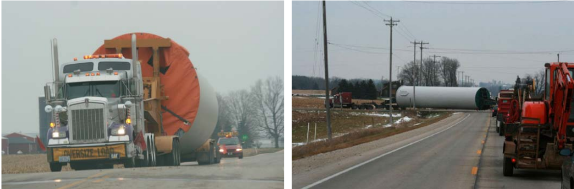
Figure 24. Difficulty in moving turbine components on existing rural roads.
